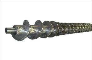
Industrial Hardfacing, Inc. offers new manufacture or complete rebuild of worn twin screws, thus restoring performance requirements.
